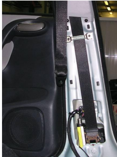
Figure 7 Seat Belt pre-tensioner during the installation
