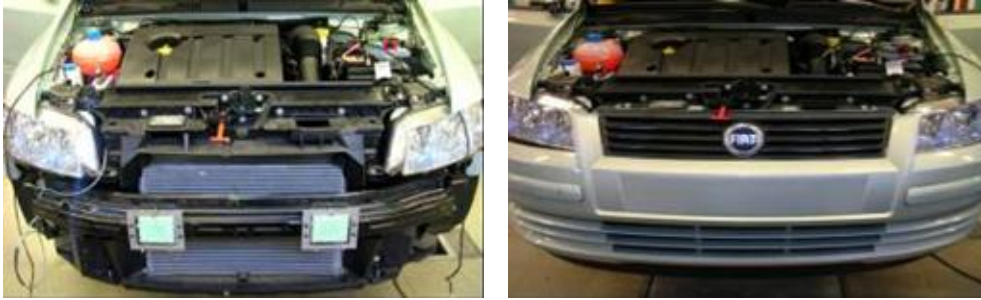
Figure 10 Front part of the vehicle during the set-up of the radar sensors and after the sensor installation
